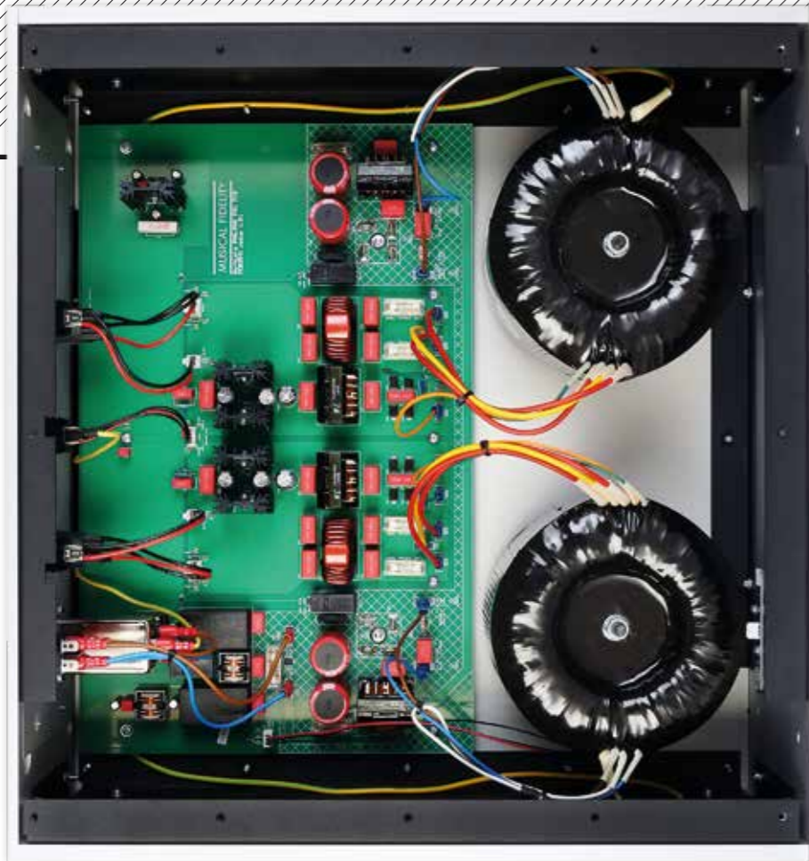
ABOVE: Inside the PAS PSU there is 'soft' rectification only. Two huge transformers [right] supply filtered 58V AC as a high-current feed (via Neutrik-terminated umbilicals) to the PAS transistor power amp stage and 12V discrete-regulated DC (via the XLR umbilicals) to feed the nuvistors' heaters
