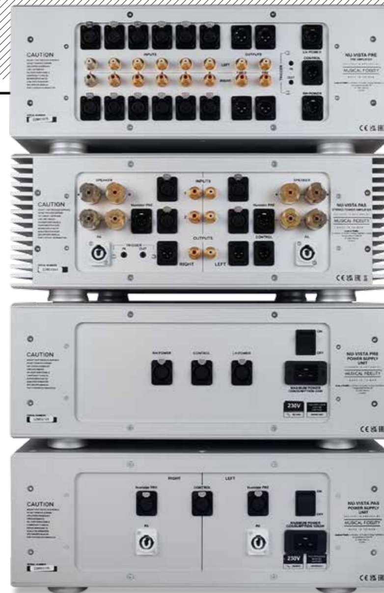
ABOVE: The PRE [top] has 12 line ins (6x RCA and 6x XLR), fixed and variable outs (on RCAs and XLRs), and control plus PSU ins for the L/R channels fed from the PRE PSU [third box]. The PAS PSU [bottom] has control plus high/low-level PSU connections for the PAS's nuvistor and power amp stages. The PAS [below PRE] has 2x RCA and XLR inputs, buffered line outs on RCA/XLR and pairs of heavy-duty speaker cable terminals
