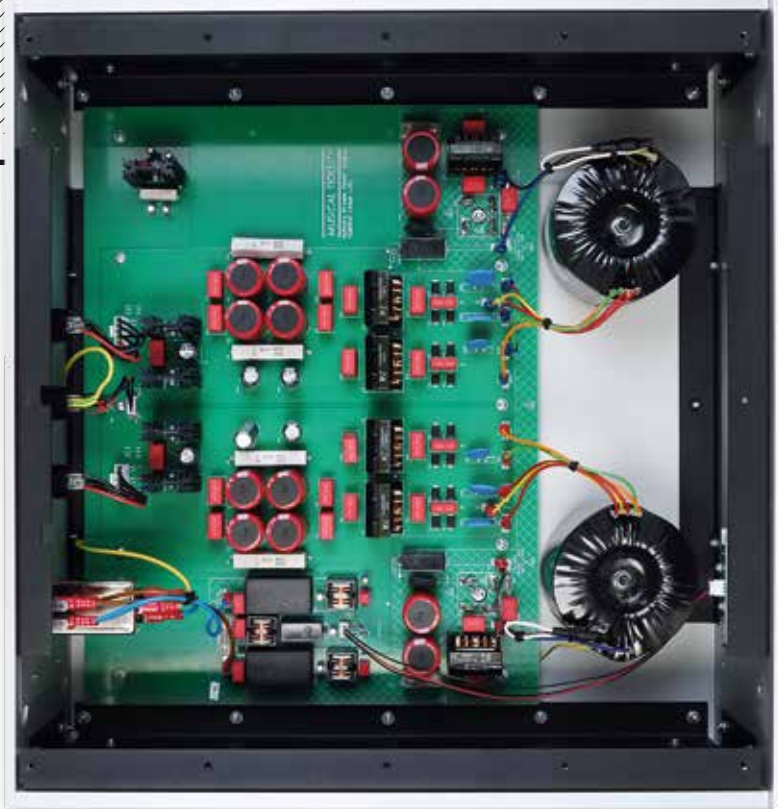
ABOVE: Inside the PRE PSU there is comprehensive AC mains filtering [centre], full rectification and regulation plus additional filtering of the \pm 55V DC feed (via XLR terminated umbilicals) to the PRE's nuvistor and transistor output stages
