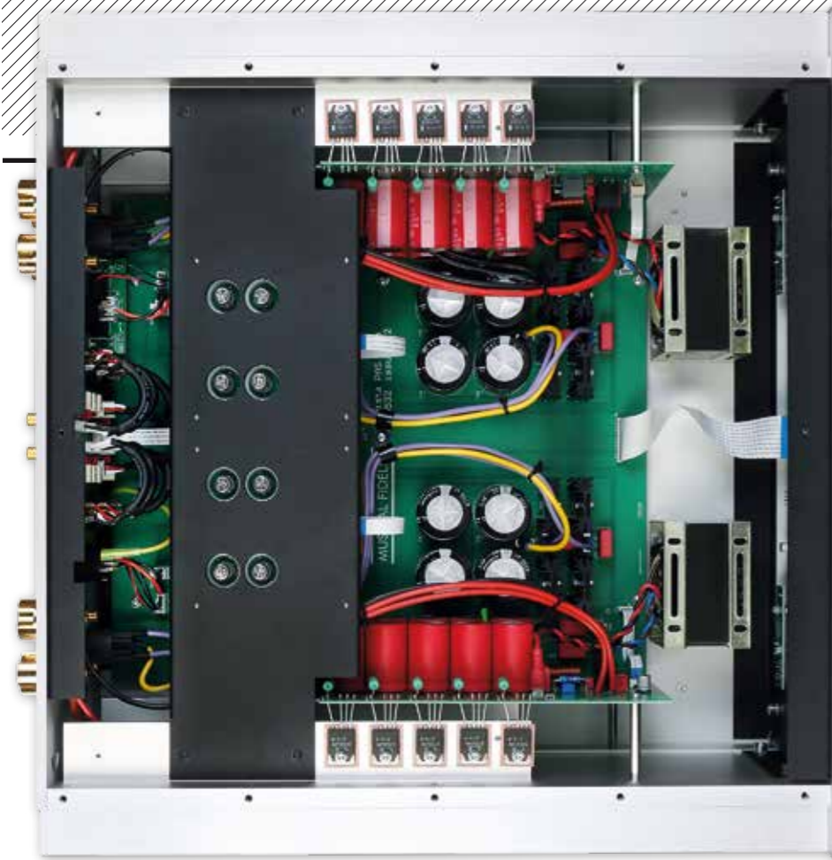
LEFT: Inside the PAS, the frame transformers [right] are common-mode DC chokes – a feature of MF's PSU regulation. Pairs of 6S51N nuvistors [left] drive five complementary pairs of Sanken output transistors per channel [top and bottom]
