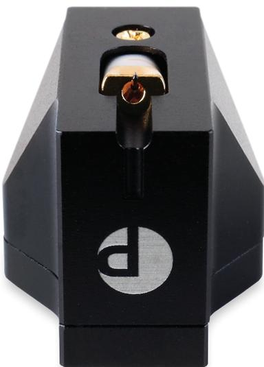
**ABOVE:** As the boron cantilever emerges from the MC9's front yoke, the 'pure iron' cross coil and 6N copper windings are just visible behind
