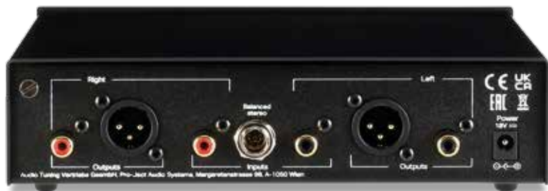
ABOVE: The Phono Box S3 B has single-ended RCA inputs and line outputs, plus balanced line outputs and a mini-XLR balanced input INSET: The X2 B turntable now has a corresponding mini-XLR output
