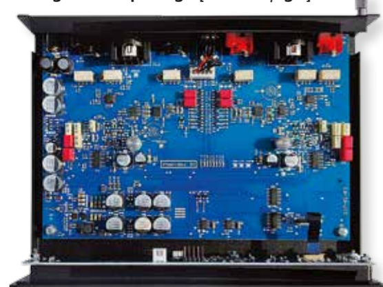
RIGHT: With the 2kg acrylic platter removed, the X2 B's sub-platter, belt and AC motor (with TPE suspension) are all revealed beneath BELOW: The Phono Box S3 B's RIAA network uses discrete transistors [left/right] but JRC2068 and NE5534 op-amps are employed in the bal. and single-ended input stages [centre left/right]
